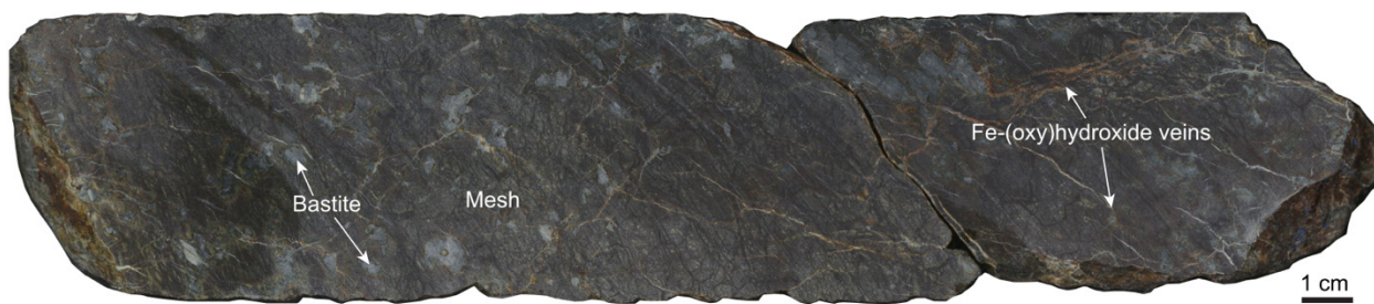
5 Fig. S14: Highly weathered and serpentinized peridotite. Fe-(oxy)hydroxide veins locally reuse former serpentine veins and cut through the serpentine-magnetite veins (mesh network) and bastite suggesting weathering postdates serpentinization (Interval 399-U1601C-27R-1, 28-55 cm).
